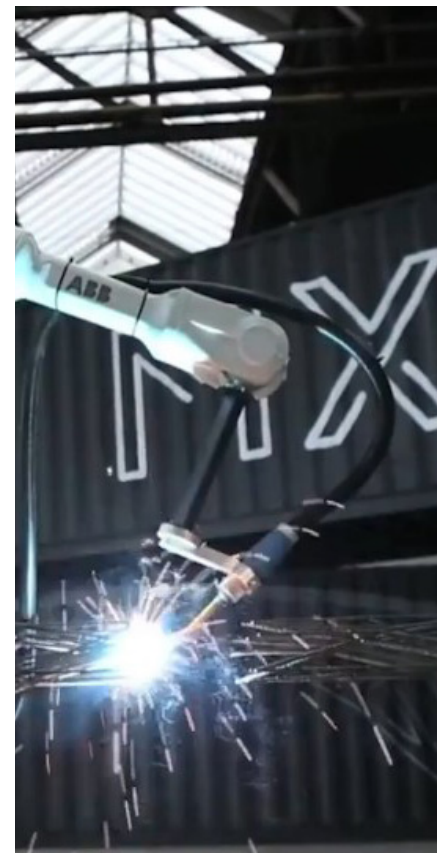
Fig.2 - Braço robótico a soldar objecto metalico, MX3D Bridge, 2017. (mx3d.com, 2017, 8)
