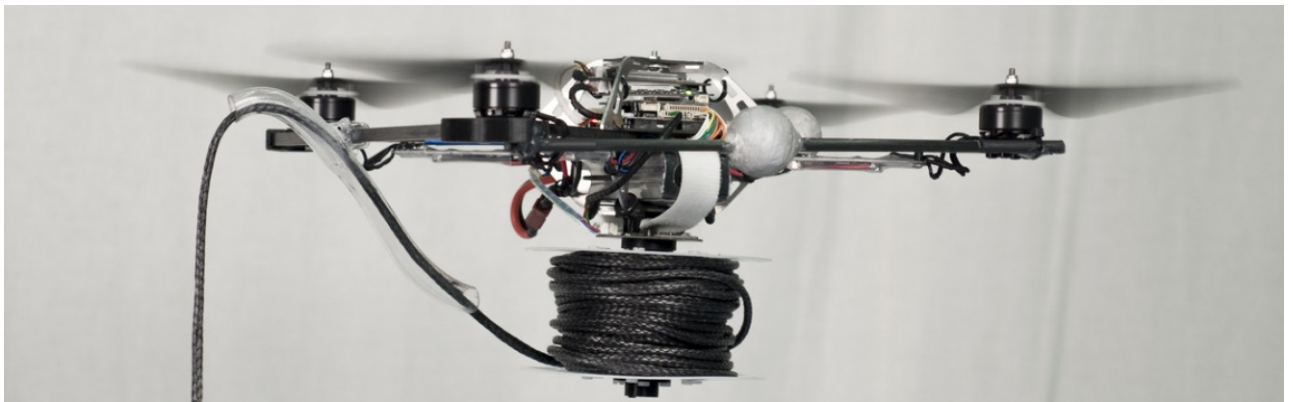
Fig.75 - Drone com carrinho automático, Aerial Construction, Federico Augugliaro, Prof. Raffaello D'Andrea, 2012. (idsc.ethz.ch, 2017, 9)
