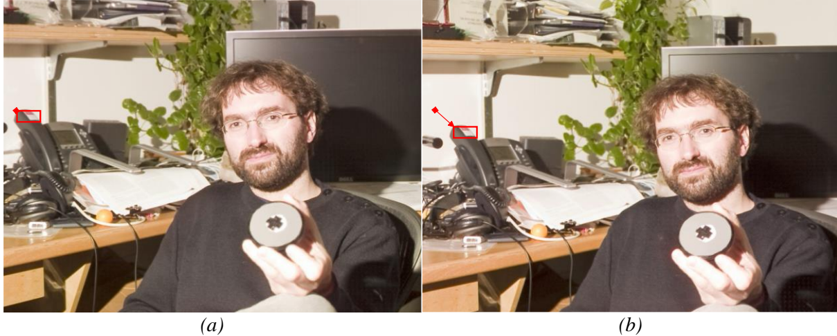
Figure 2.13 Comparison of two 2D views rendered from the LF test image Fredo (see Figure A.1) using the Weighted Blending algorithm with two different patch positions (relative to the MI center): (a) (-18, -18) ; and (b) (18, 18) . The disparity of the captured phone in the two views is highlighted by a red arrow.
