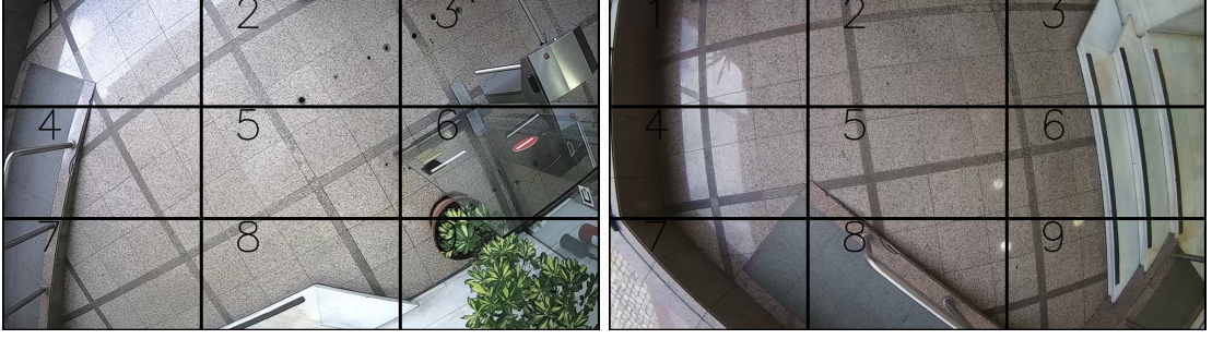
Figure 4.3: Grids drawn over camera fields of view. These grids enable us to define static rules about which trajectories are possible and which trajectories are not, which is useful for the system to recover from diverse tracking errors.
