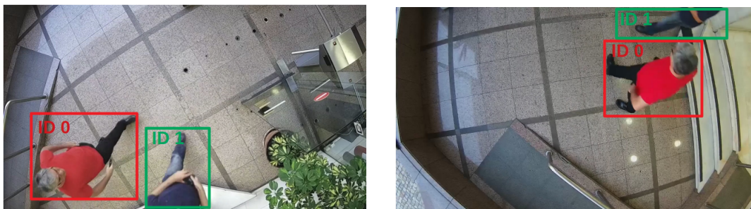
Figure 5.1: Multiple Camera Tracking: camera feeds should be perfectly synchronized in time and the same objects in the different feeds should be linked together in one single trajectory with one object identifier.
