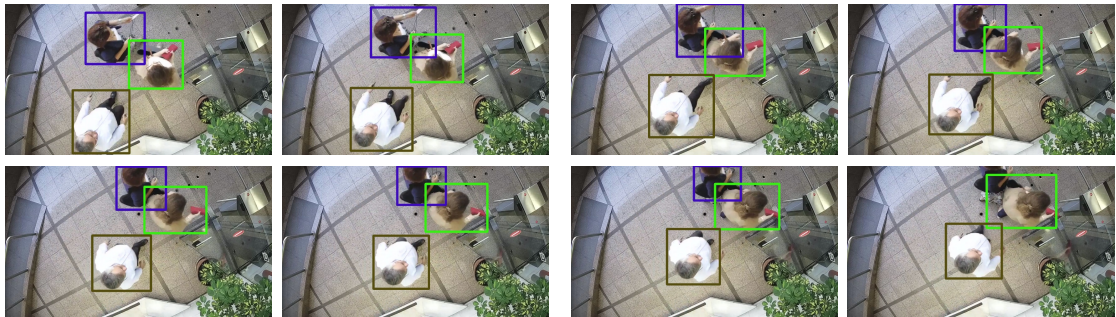
Figure 6.16: Tracking sequence example— Predictions made by the GOTURN tracker with an IOU Affinity Measure.
