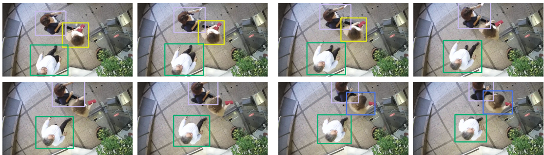
Figure 6.18: Tracking sequence example—Predictions made by the Deep Sort tracker.
