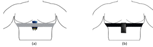
Fig. 2. Prototypes for RR Estimation. (a) BMA400 Accelerometer attached to an Elastic Band. (b) Proposed Prototype based on Pressure Sensor Mechanism.
