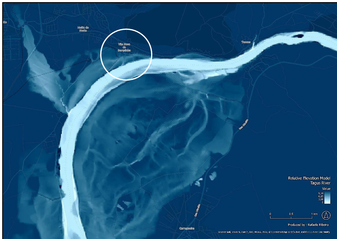
Figure 10 – Relative Elevation Model (REM) of the Tagus River in the Vila Nova da Barquinha area, obtained from a Digital Terrain Model (DTM) and the modelling of the river channel surface. The REM represents the altimetric difference in relation to the riverbed (value 0), allowing the identification of variations in the alluvial plain, such as flood-prone areas and fluvial terraces. The altimetric database used for the calculations in the ArcGIS software was provided by the Direção-Geral do Território (DGT) and made available by Esri. © Rafaela Ribeiro, 2026
