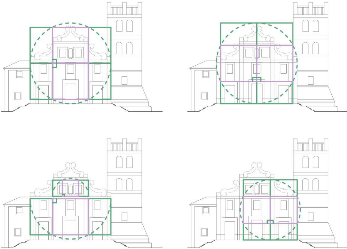
Fig. 8 - Modulation of the façade of the Church of Matriz; Prepared by Vieira
