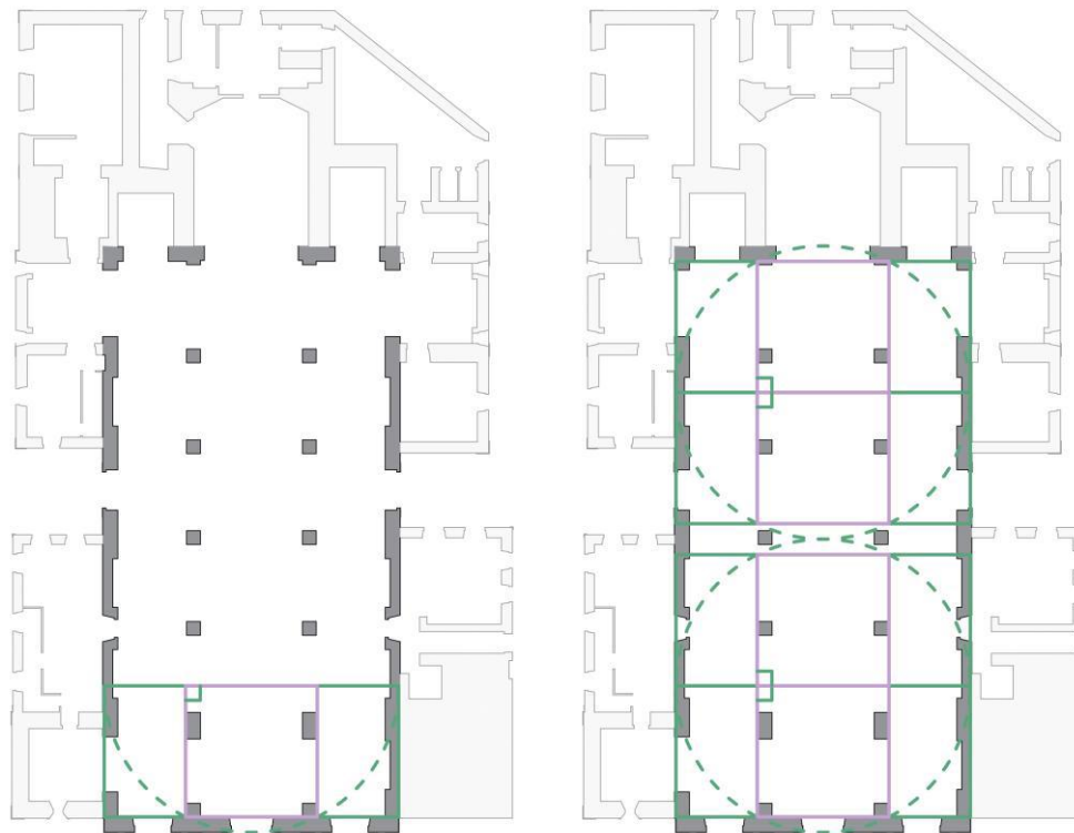
Fig. 4 - Superimposition of the modules in the Church of Matriz: (left) rectangle with a \sqrt{5} side; (right) its multiplied form ( 2\sqrt{5} rectangle); Prepared by Vieira
